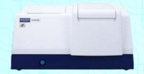
Optical system: Double beam monochromator
